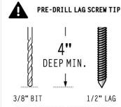
USE A 3/8" BIT AND PRE-DRILL AT LEAST 4" DEEP BEFORE INSTALLING 1/2" LAG SCREWS.
