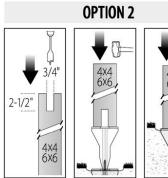
Drive Load Fin with hammer and post block.
