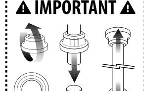
Collars have Inner Male ALIGNMENT COLUMNS Align COLUMNS with Female opening
