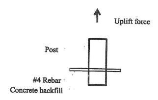
½" diameter (#4 rebar) Check wood crushing  $F_c$ ' =  $F_c$   $C_M$  = 525 psi
