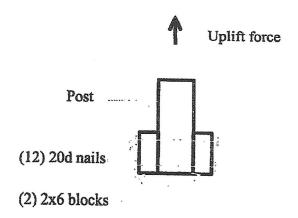
2x6 block on both sides of post (6) 20d galvanized nails per block (each side) Nail capacity in shear,  $z' = z C_D C_M = 152 lbs (1.6)(0.7) = 170 lbs$
