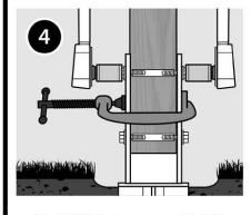
Use TWO Ratchets and 9/16" Sockets to *Tighten* Cap Screws and *Secure* Post.
