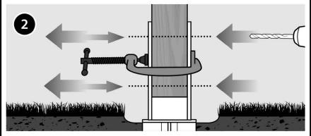
Drill through CENTER HOLE, POST and out the OPPOSITE HOLE.
