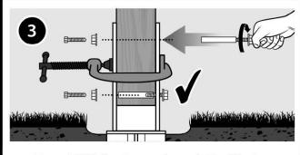
Thread ONE Cap Screw through Hex Washer partially into Coupling Nut. Insert Screw and Nut into Post. Thread OTHER Cap Screw with Hex Washer into Coupling Nut.
