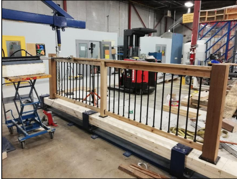
Photo No. 1 Horizontal Top Rail mid-span Load Test
