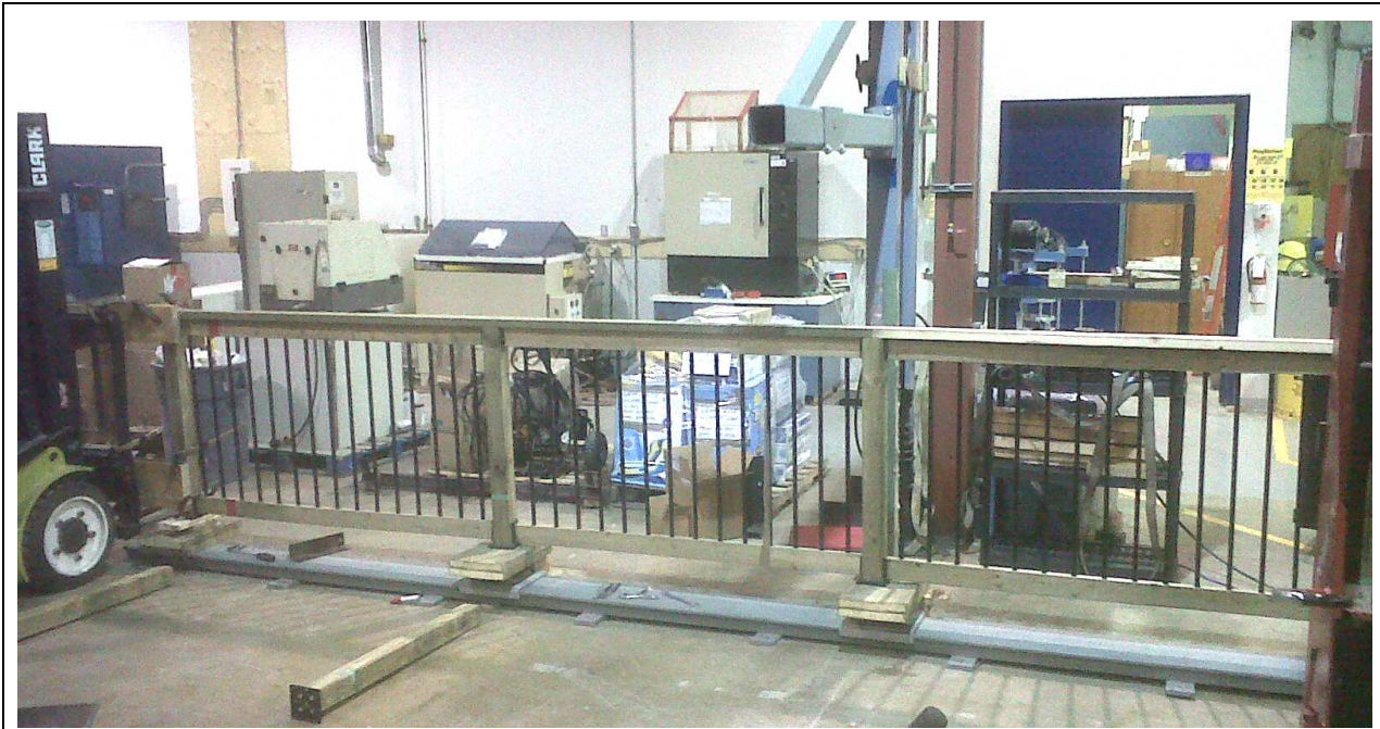
Photo 1. Guard Rail system (Top Railing Option 1) being tested. The post on the left side is completely fixed to the forklift. All the other posts are cantilevered from the ground.
