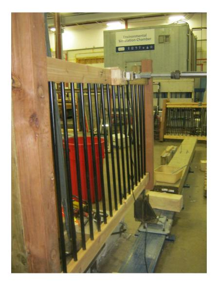
Photo 1 Top Rail Loaded at Midspan
